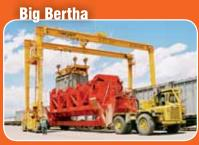
**Versatility** - Big Bertha employs a unique dumping mechanism that provides structural support to allow container rotation of 150° while maintaining the integrity of the unit.
