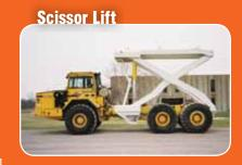
**Landfills** - Eliminate the transfer station! The PHIL Scissor Lift can be configured to carry your container and dump directly in a railcar or other mode of ongoing transport.
