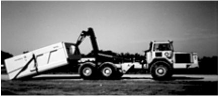
Figure 4.2. Picking Up/Dropping Off A Roll-Off Container
