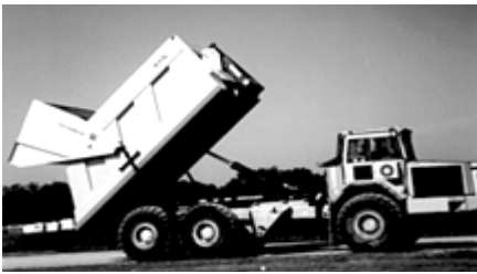
Figure 4.4. Opening of the Roll-Off Container Autogate ®
