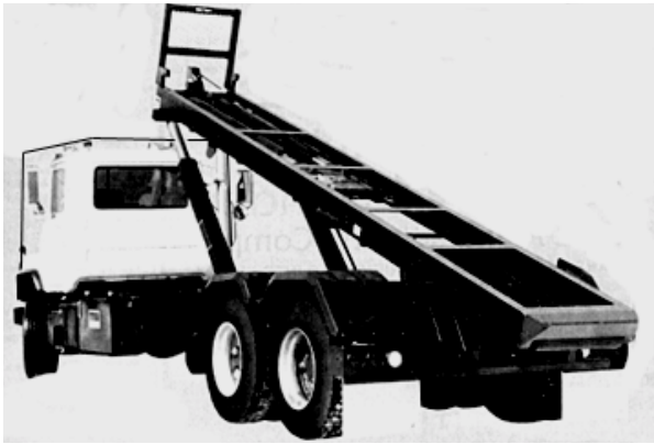
Figure 2. "Winch" Based Roll-Off Container Transport Truck
