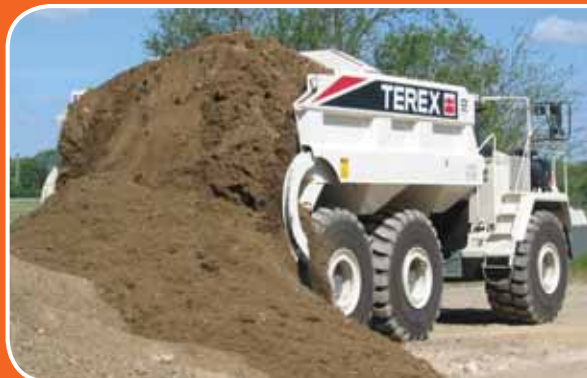
Rear Eject body ejecting load.
