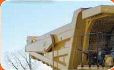
Sideboards are recommended to increase volumetric capacity when hauling lightweight material and when loading height is not restricted in situations where custom truck bodies are not a practical alternative.
