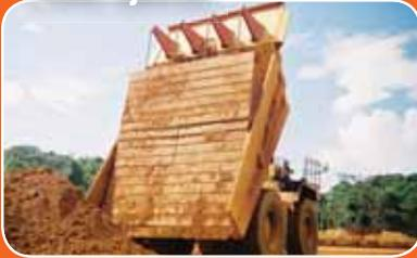
The PHIL Load Ejector dislodges sticky material clinging or sticking to the truck body through a series of overlapping, jointed steel plates attached to the top of the front slope plate and extending down the body floor. In the dump cycle, the Load Ejector slides away from body floor, hanging vertically or nearly vertically, to dislodge sticky material.
