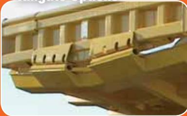
**Rubber Cushion Pads** are recommended for underground operations and operations with high road speeds or uneven haul roads. Shown at left, Cushion Pads reduce wear, bouncing and noise and often increase the life of your PHIL Autogate® Tailgate. These may be installed on an existing gate or purchased with the tailgate.
