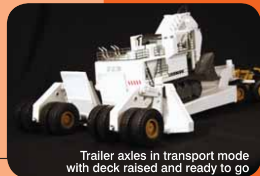
Ramps up, trailer axles ready to swing into transport mode
